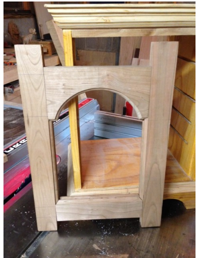
My first success in cherry, you cut the horns after the door is glued up.
