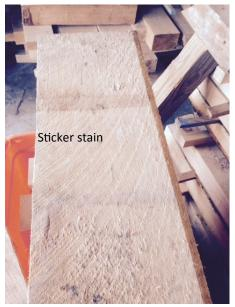
Typical rough sawn cant of basswood this piece came off of a circle mill. The dark lines on the cant are sticker stains used in the drying process and discolorations that will plane out
