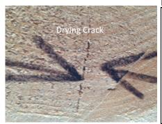
Here are a couple examples of end grain checking, caused during the log drying as you can see they can be hard to see. In logs I try and seal the ends with a special paint that minimizes end checking but some still occurs. Something to look for and plan your cut out with it in mind. I remove this when I see it but once in a while it is missed
