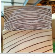
Sometimes two chunks of wood the same size can weigh different. Some wood is denser this can make it a little harder to carve but it holds detail better and some folks look for that. The top chunk was 3/4 pound heavier but the rings on the heavier piece were very tight the chunk on the bottom were farther apart
