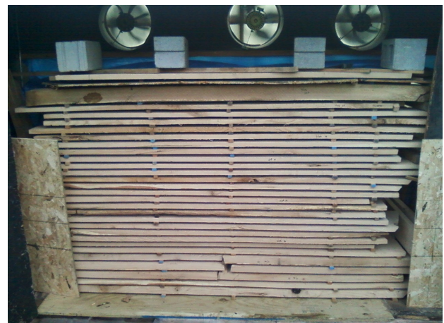
Red oak that is in the process of drying it is currently about 16% so it still has a ways to go yet. The fans circulate the warm air and remove the moisture. The cement blocks help-keep the lumber pile from warping.
