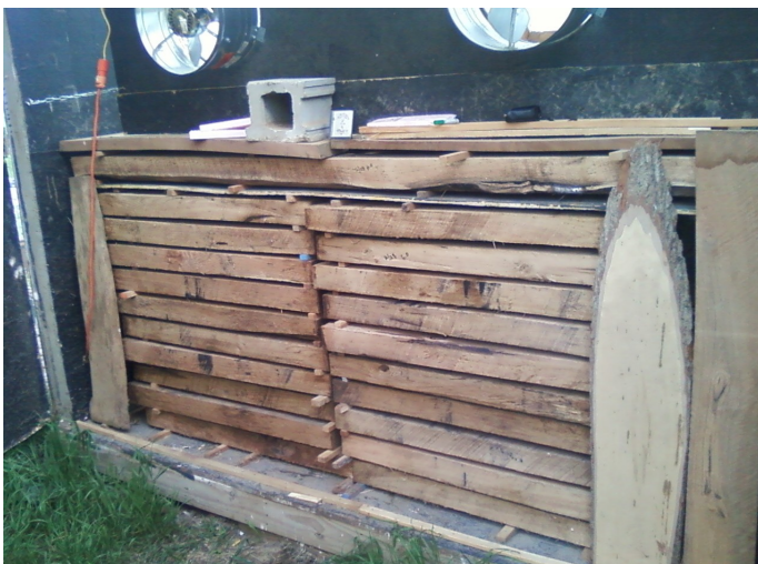
A load of butternut in my kiln, dry and ready to stack as soon as I can find a place to stack it. The inside of the kiln is painted black to increase the kiln temps.
