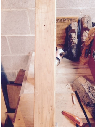
This is just a 2X4 that you can attach the bark to with screws from the back
