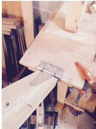
It is attached with a hinge and then clamped to my bench
