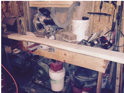
Using a sliding saw the blocks are cut to yield the best amount of clear stock
