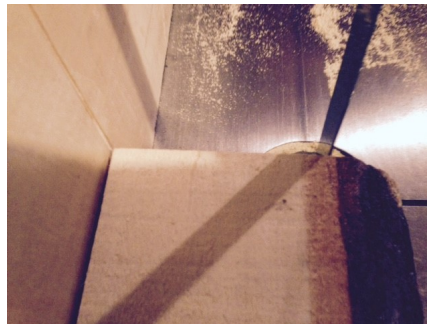
The blocks are then ripped on the bandsaw to remove defects as needed
