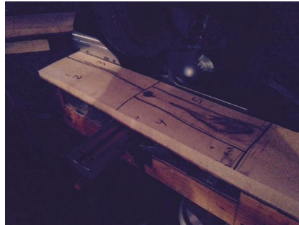
Using a sliding saw the blocks are cut to yield the best amount of clear stock
