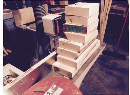
Once the blocks are cut I joint one edge for a straight reference for the next step.
